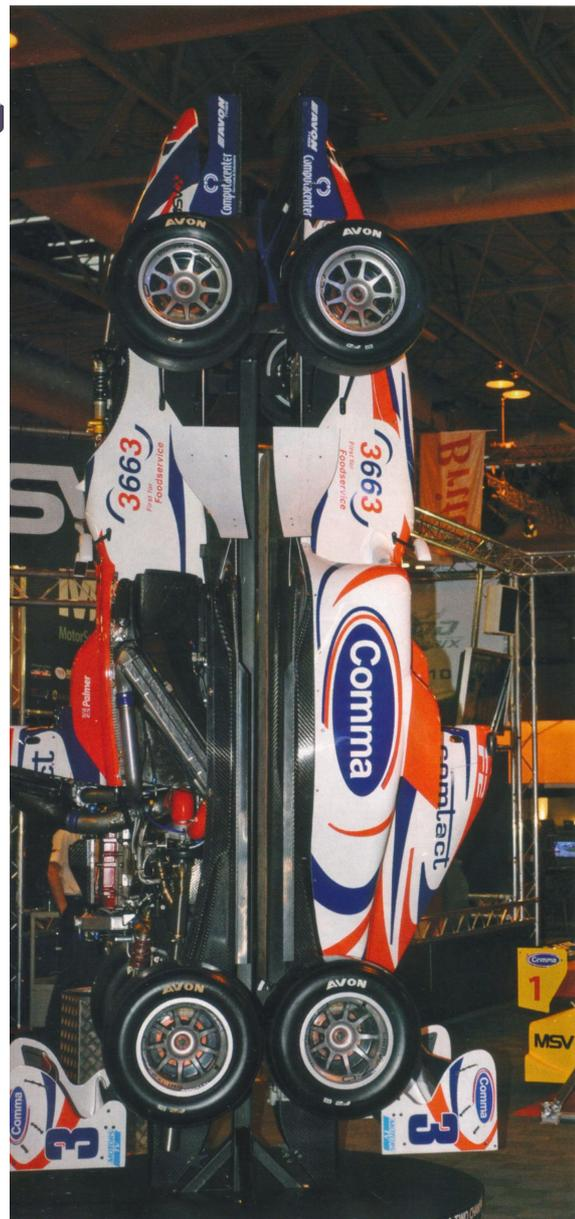
A steel column support for two Formula Two racing cars suspended vertically, via precision laser cut plates designed to support the suspension wishbones. The support was designed for both crowd loading during the show and installation loads when the structure would be eccentrically loaded by only having a single car suspended from the support.
